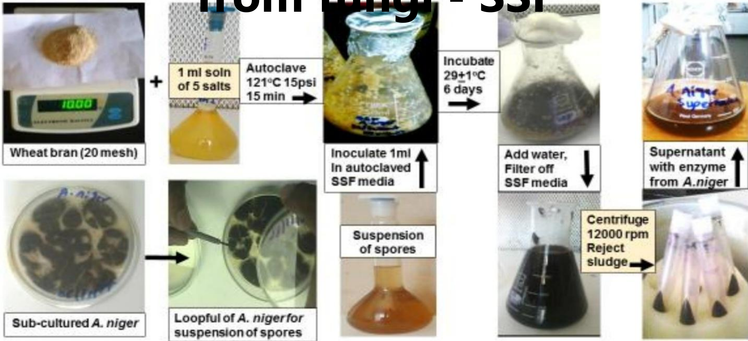
Fig. 1 Steps of Solid State Fermentation process to obtain enzyme from the fungus Aspergillus niger
