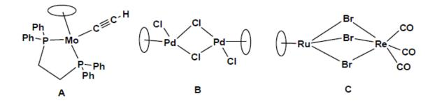
5. Four chlorine ligands are missing in each of the given skeletons of dimeric compounds A, B and C. Given that all of them obey the 18 electron rule and no additional metal-metal bonds are present, attach the missing Cl ligands on the complexes in the most appropriate manner.
