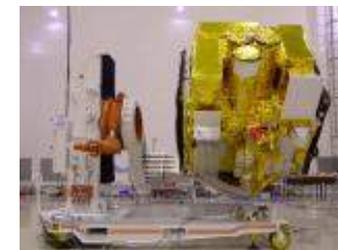
*ASTROSAT in tilted position in clean room for a pre-launch test*
