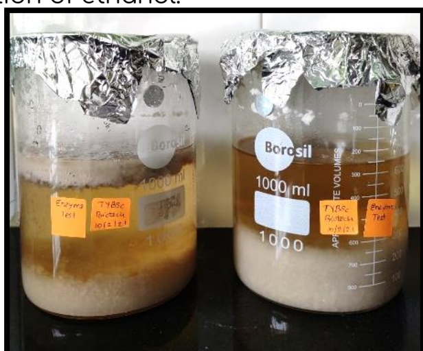
Fig. L-R: .Enzymatic hydrolysis treatment of cellulosic substrate i.e.tissue paper and Distillation of the substrate slurry after anaerobic fermentation for production of bioethanol
