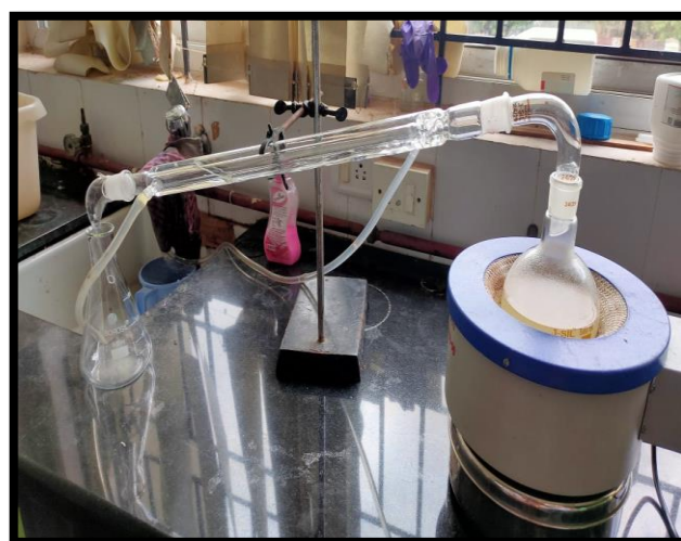
Fig. L-R: .Enzymatic hydrolysis treatment of cellulosic substrate i.e.tissue paper and Distillation of the substrate slurry after anaerobic fermentation for production of bioethanol
