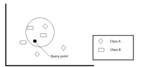
The distance between the test data point and the training data point is found out with the help of the Euclidean distance formula:
