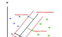
Non-linear SVM: For nonlinearly separated data non-linear SVM is used. In other words if a dataset cannot be classified using a straight line, then such data is called non-linear data and the classifier used is called the non-linear SVM classifier. Kernel function transforms the set of data so that a non-linear decision surface is able to transform to a linear equation in a higher number of dimension spaces.
