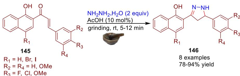
Scheme 17. Solvent-free synthesis of 2-pyrazolines (**146**) using grinding technique [180].
